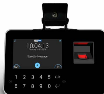
Example of MITO-03 installed on X3 BIO terminal
