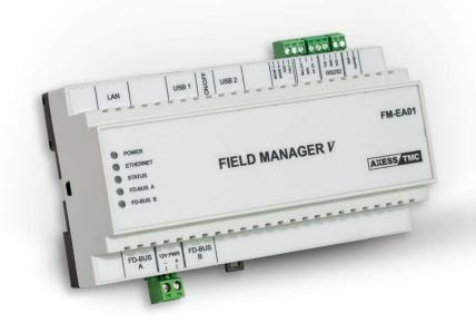
The Field Manager device allows distributing the intelligence of the access control system, ensuring the functionality of most advanced Independent Servers. The Field Managers are intelligent multi-application units equipped with a stand-alone database that is updated online by the XAtlas software. The devices can automatically execute all the field processes relating to different applications such as access control, intrusion detection and time and attendance.
