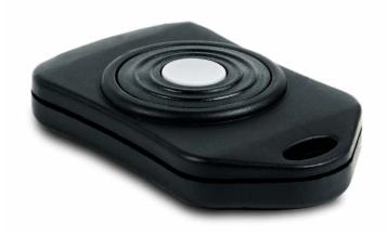
BLETag is a pocket Bluetooth Low Energy transponder: an active Tag with lithium battery based on BLE technology. BLE is a wireless communication technology that, unlike conventional Bluetooth, does not require preliminay «pairing» between devices. Taking advantages of BLE flexibility, we developed an active tag suitable for tracking people and items.
